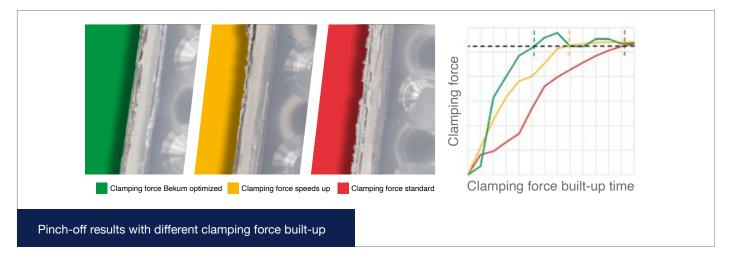
The new Bekum clamping system (e-Twin-Toggle) builds the necessary clamp force up in < 100 ms, thus, the EBLOW 807D is particularly well-suited for the production of PP handleware bottles.
