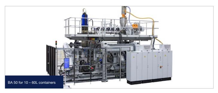
The BA 50 has now bridged the gap between the BA 34.2 canister machine for up to 30 I and the large blow-moulding machines for 60 I or more.
